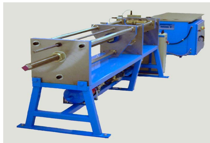
25 + 2 kip Dual Test Frame With HPU
