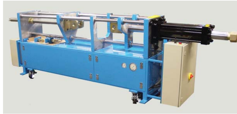
75 kip Integral HPU Test Frame
