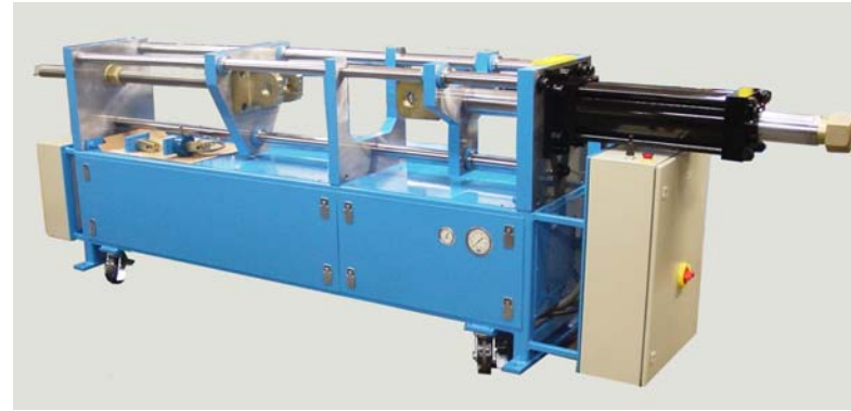
75 kip Integral HPU Test Frame
