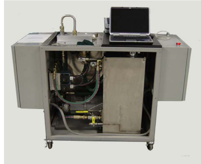
Valve Test Machine for Paul Munroe/Enertech Snubber Valves
